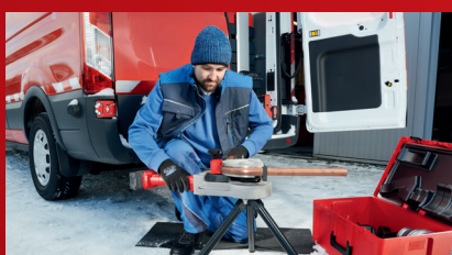
Pre-adjustment of the bending angle without tools
