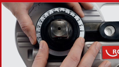
Pre-adjustment of the bending angle without tools
